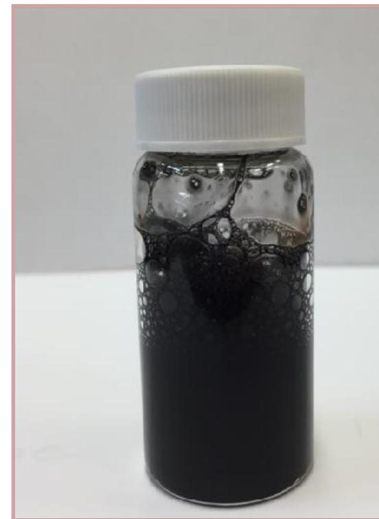
Graphene suspended in 0.5% of BSA solution, concentration of graphene 1mg/mL
