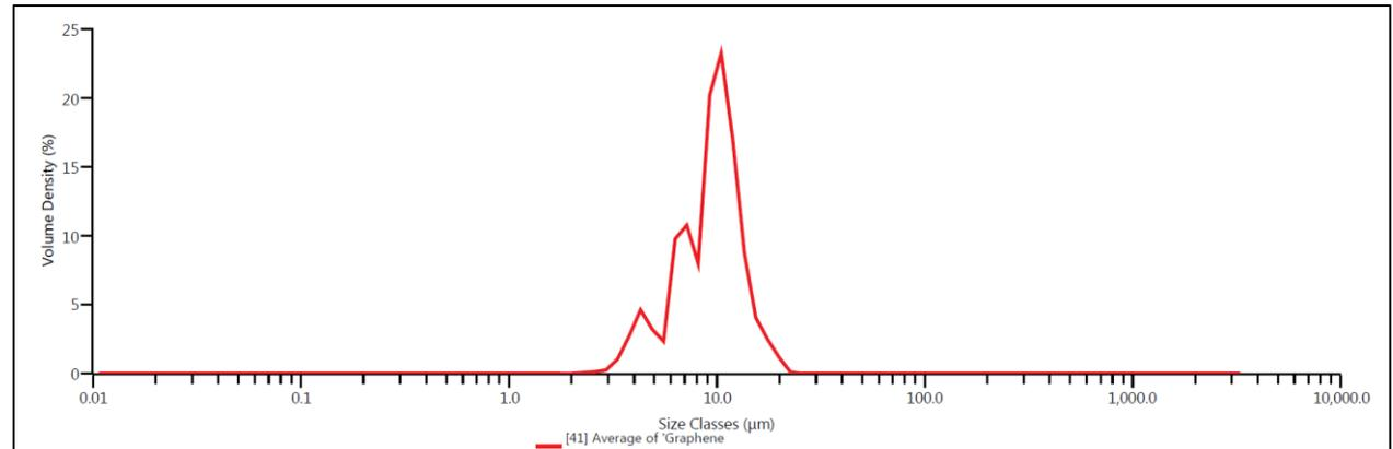
Histogram of Microfluidized graphene in injectable water
