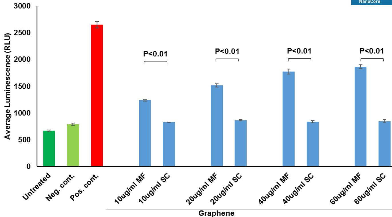
**TF 9-2 ROS-Glo™ H2O2 Assay (Non-Lytic Assay)** signals from LLC-PK1 cells exposed to graphene (microfluidized; MF and sonicated; SC) for 48h, cells treated with injectable H2O was used as a negative control; Neg. cont. and 50 uM menadione in medium was used as a positive control; Pos. cont.
