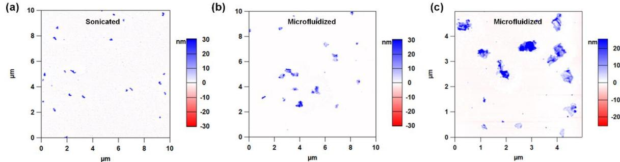
**Figure 2.** (a) Representative morphology of sonicated graphene surface. (a) Microfluidized graphene sheets visualized using AFM. (c) A zoomed in image of the same sample with microfluidized graphene.
