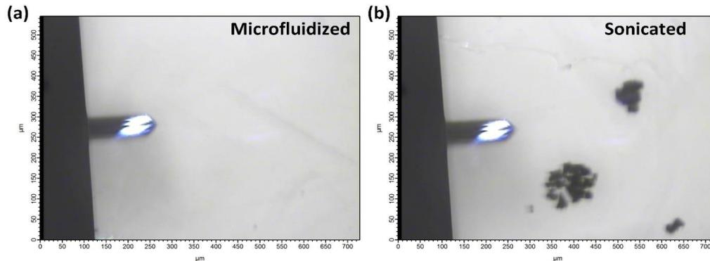
**Figure 1.** Graphene sample surface visualized through the AFM video camera. Representative sample areas are shown for (a) microfluidized and (b) sonicated graphene sample. The surface distribution of graphene looked significantly different when observed through the AFM video camera image.
