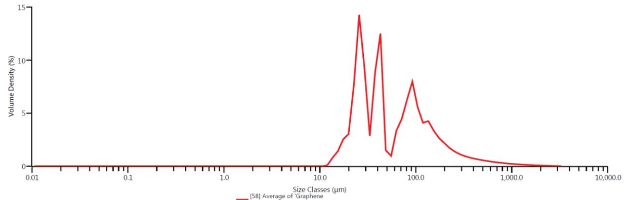
Histogram of Sonicated graphene in injectable water
