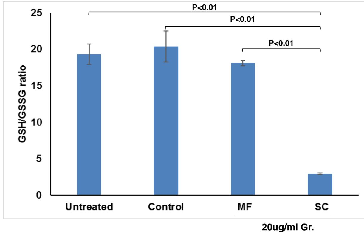
TF10-1 Reduced glutathione/Oxidized glutathione (GSH/GSSG) ratio in LLC-PK1 exposed to graphene (Gr.) dispersions prepared by sonication (SC) and microfluidization (MF) methods for 24h by using GSH/GSSG-Glo™ Assay
